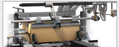
Flap folding (not plowing) and positive case squaring
