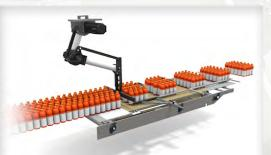
Smartrak<sup>®</sup> Mass flow infeed design eliminates soft bottle bridging and removes gaps to ensure pack pattern accuracy and continuous product flow.
